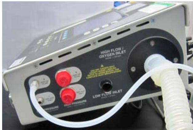
Pneumatic connections with the calibration device (VT-Plus)
