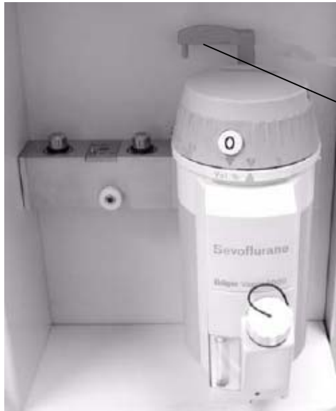
Locking Mechanism Handle in the locked Position
