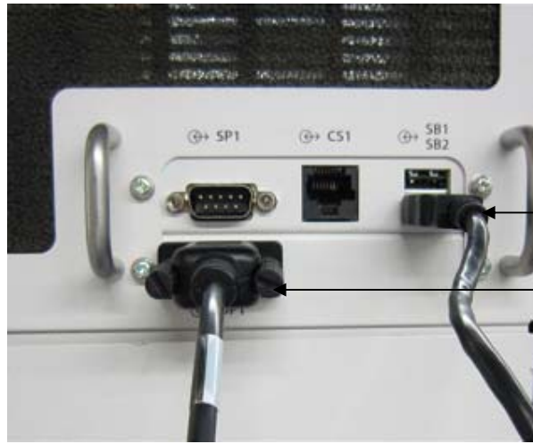
Cable connections at the anesthesia machine end
